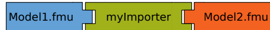
Figure 1. Co-simulation approach of the FMI standard (a framework approach): The standardized FMU models are called and coupled by an importer program. We denote the caller (executable) with a female connector and the callee (library) with a male connector.
