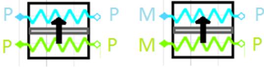
Figure 3. Boundary condition types: pressure - pressure (left) and Mass flow rate - pressure (right).
