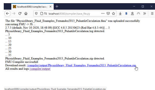
Figure 4. Bodylight FMU Compiler - web form showing process of compiling FMU to JS packed as ZIP archive
