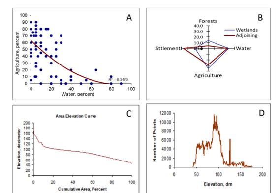
Figure 6. Analysis of wetlands habitat based on physical data: A. Wetlands agriculture and water persistence relationship; B. Proportion of agriculture lands, waterbodies, forests and settlements; C. Area Elevation Curve; and D. Land elevation histogram.
