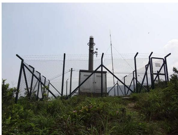
Figure 1. CORS ground station with security fence – Ngong Ping Station – Hong Kong
