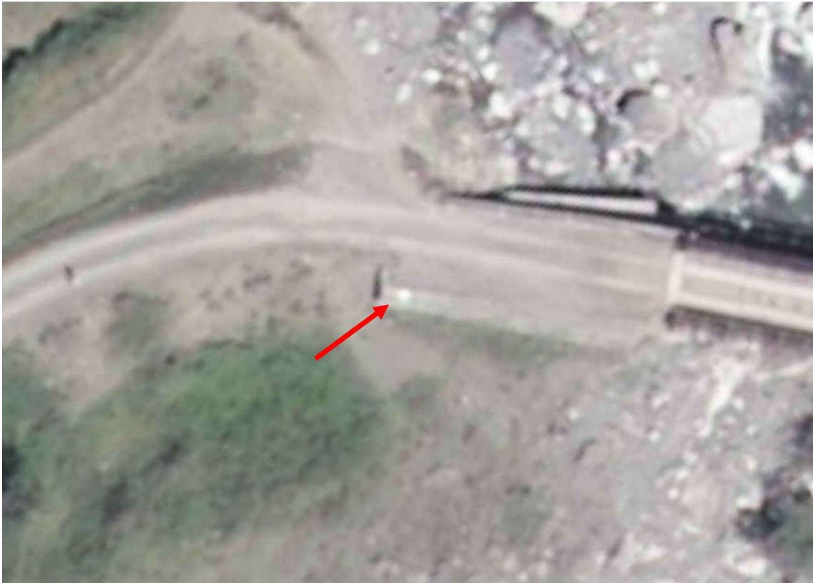
Figure 7: Ground mark shown in Figure 6 visible in an aerial image with 30cm ground resolution (source Hansa Luftbild AG, 2016)
