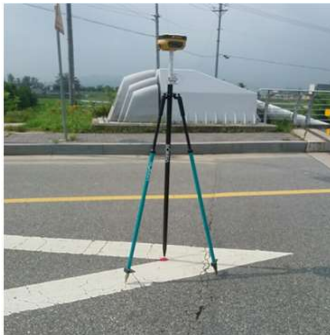
Figure 4. Placing a ground mark
