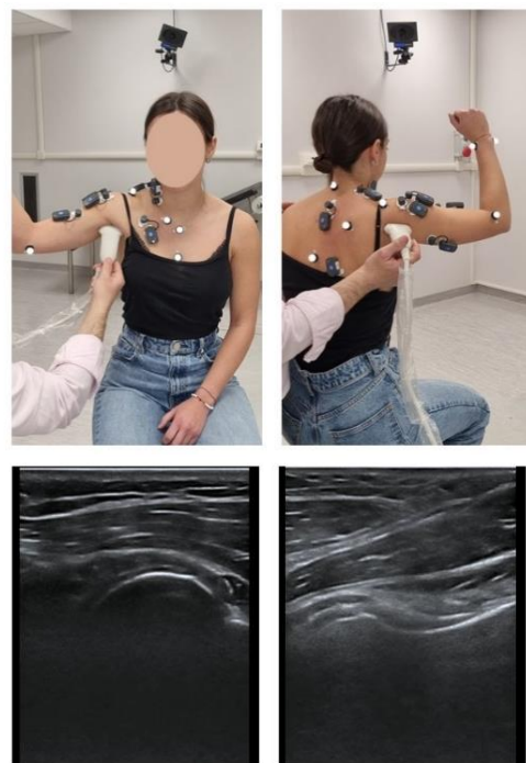
Figure 1: Experimental setup comprehensive of passive reflective markers, surface EMG electrodes and ultrasonography probe are shown (top). Examples of ultrasonography images of the humeral head from 2 probe locations (i.e., anterior axillary line and posterior aspect).
