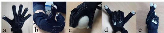
Figure 1: Postures for validation: (a) Fingers max. abduction; (b) 90° fingers metacarpophalangeal flexion and thumb max. extension; (c) Grasping a ball; (d) 'Y' from American Sign Language (ASL); (e) 'R' from ASL.
