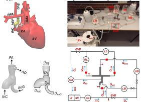
Figure 1: Schematic anatomical illustration (top-left), 3D geometry (bottom-left), and in vitro circulation loop (right) of the assisted Fontan using the proposed venous ejector pump (VEP). Red squares and dots represent flow meters and pressure sensors, respectively.
