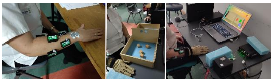
Figure 1: Subject instrumented with 7 EMG electrodes (left) while performing the real (centre) and virtual test (right).
