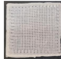
Figure 2: Fabricated PVA-C sample with an alternating 0-90^{\circ} toolpath.
