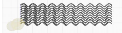
Figure 1: CAM toolpath design, based on a sine-wave.
