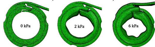
Figure 2: Wrapping capability of a specific AUS configuration - conformations at different cuff pressures.
