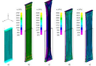
Figure 1: Distribution of 1<sup>st</sup> principal (Cauchy) stress in FE simulations of uniaxial tension test using different constitutive models: a) mesh with the applied boundary conditions, b) non-structural GOH model, c) non-structural HGO model, d) structural GOH model, and e) structural HGO model.
