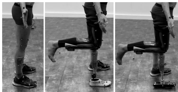
Figure 1: Illustration of the three conditions tested. From left to right: without prosthesis; with the prosthesis simulator equipped with an energy restitution foot; with the same simulator equipped with a rigid foot.
