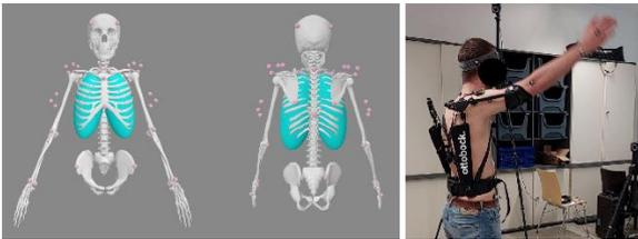
Figure 1 (left): The biomechanical model developed in OpenSim; Figure 2 (right): Arm elevation trial with the exoskeleton.
