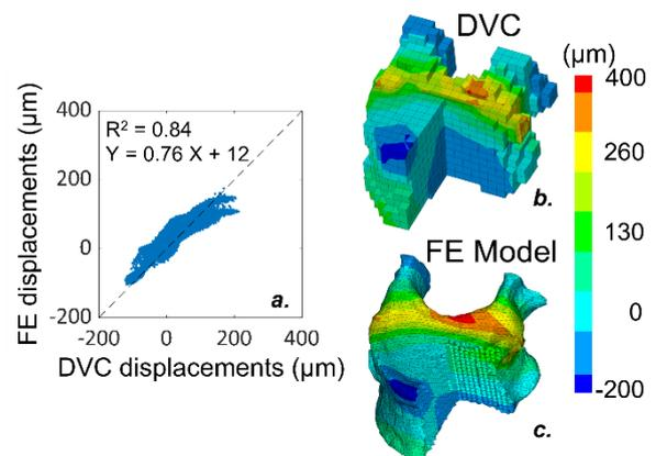
Fig.1: Scatter plot (a) between experimental (b) and numerical (c) displacements in the cranio-caudal direction for one of the control vertebrae analysed.
