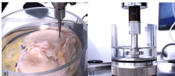
Figure 1: Experimental setup for normal indentation (a) and unconfined compression tests (b).
