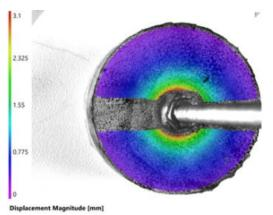
Figure 1: Indentation of a cylindrical silicone sample with displacement measurements using 3D-DIC.
