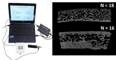
Figure 1: Osteoprobe microindenter (left); one- (top) and three-layered (bottom) bone samples
