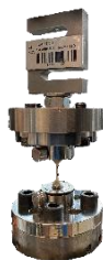
Figure 1 Experimental setup showing a cylindrical bone specimen being tested elastically in tension.
