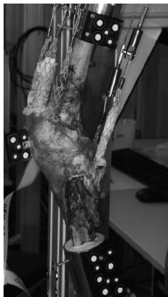
Figure 1: Knee rig with native knee and optical markers for kinematics tracking.
