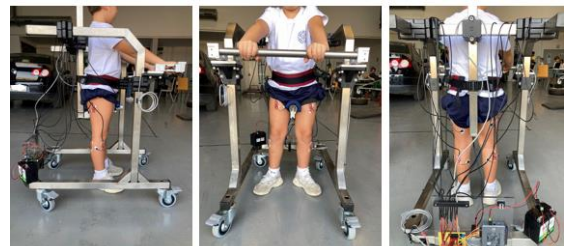
Figure 1: Sensorised child walker with subject during the experimental trial.
